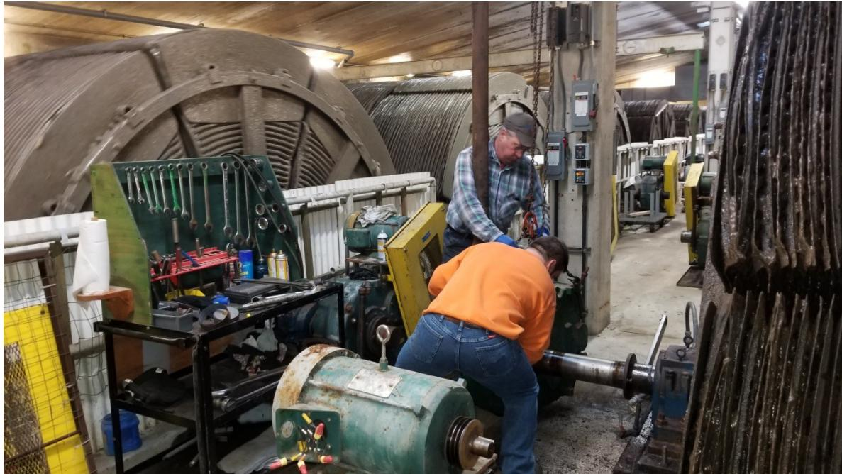
Both RBC #1 bearings were replaced successfully during the week of the 22<sup>nd</sup>. The failed bearing removal required use of an angle grinder to chop off the outer track to gain access to the cage and rollers and then the inner track had to be cracked and split in order for it to be removed from the shaft.
